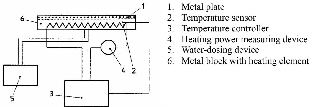
Figure 15. Measuring unit
