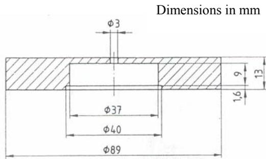
Figure 7. Calorimeter mounting block
