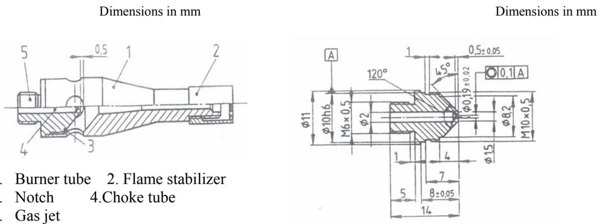
Figure 2. Gas burner
