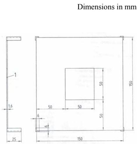
Figure 9. Specimen support frame
