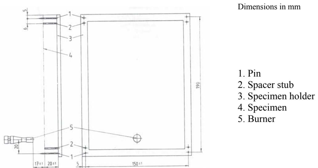
Figure 1. Mounting frame
